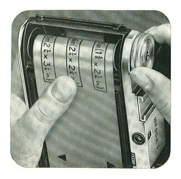
Now turn the film winding knob until the two arrow heads ◀▶ on the backing paper come into view. Close the camera back, and make sure that both catches engage properly.
