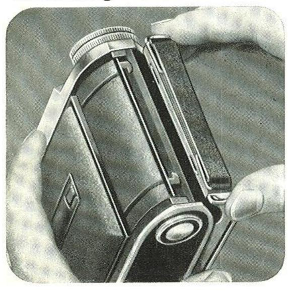
The Bessa I has been purposely designed to take only roll film spools having a thick core of metal or wood, and marked on the packing with B II/8 or 120. You obtain 8 exposures of  $3^{1}/_{4}\times 2^{1}/_{4}$  inches each with these films, or, with the film mask, 16 exposures of  $2^{1}/_{4}\times 1^{5}/_{8}$  inches  $(4.5\times 6 \text{ cm.})$  each.
